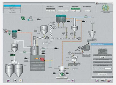
• DCS (*Distributed Control System*) used for continuous processes control. The main requirement to such systems is fault tolerance. High fault tolerance is achieved by backup of software and hardware elements of the system, use of high-reliable components, implementation of comprehensive diagnostic facilities and maintenance and constant human control.
